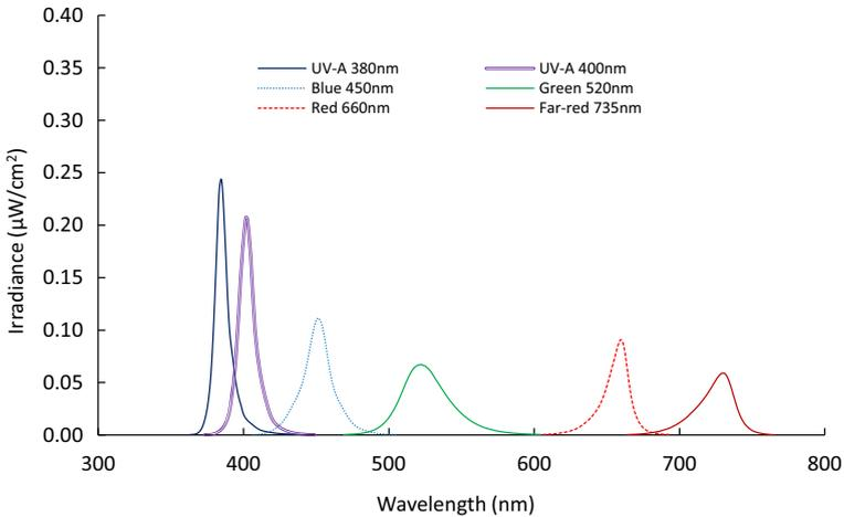
**Fig. 1** Spectral distribution of light-emitting diodes with different wavelength maxima (RX-30, Heliospectra AB, Sweden) used in the experiments
